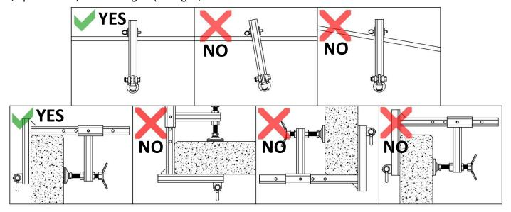
Figure 4 – Proper Orientation view of Parapet Anchor
