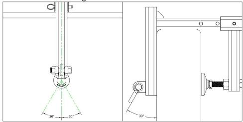
Figure 2 – Parapet Anchor Angular Limitations
