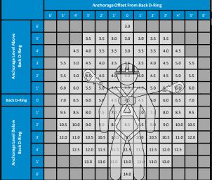
Clearance required between working surface and nearest obstruction in feet. Note: Includes 2 ft. safety factor.
