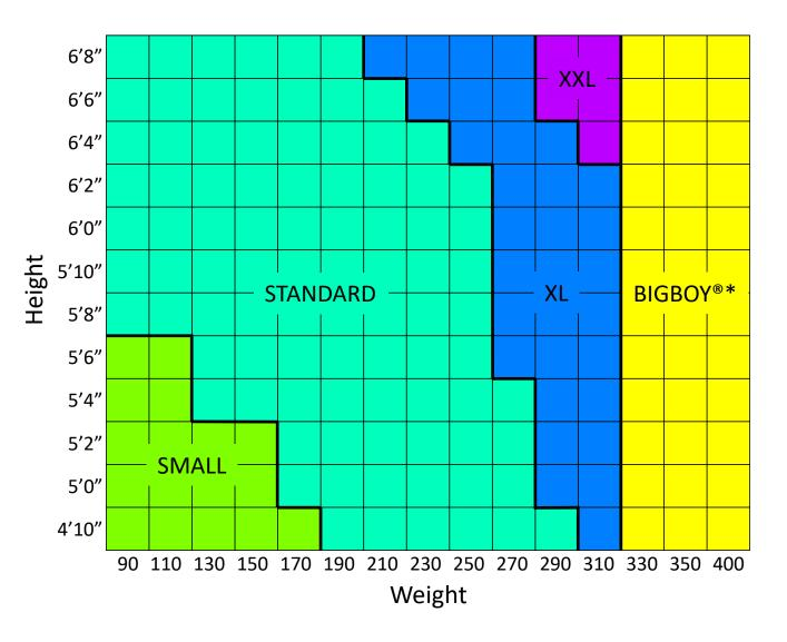
Reliance Fall Protection full body harnesses are manufactured and rated to comply with the requirements of all applicable ANSI standards. ANSI Z359 recognizes the use of full body harnesses only within a user weight range of 130 to 310 pounds.
