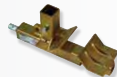
6235 - HLL Stanchion Inverted Beam Clamp fits 4 1/2" - 14" width 1/2" - 1 1/2" thick (11.4 - 35.5cm width 1.2 - 3.8cm thick)
