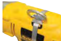
REL799971 Light / REL799973 Heavy Rings For tools up to 20 lbs (9kg) [REL799971] & 50 lbs (23kg) [REL799973] that have no adequate means for connecting the tool lanyard. REL799971 installed using the REL799960 3/8" (9.6mm) banding; REL799973 installed using the REL799962 1/2" (13mm) banding. (sold in pks of 10)
