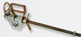
3092 - HLL Foot Rest Beam Clamp fits 4" - 16 5/8" width 1/4" - 1 3/4" thick (4 - 41.5cm width .6 - 4.4cm thick)
