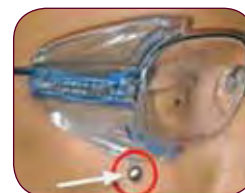
A B-26 Side Shield successfully deflecting a 1/4" steel ball at 150 fps (102mph) during testing.
