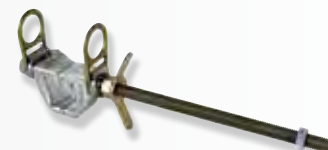
3098 - HLL Double End Anchorage Beam Clamp fits 4" - 16 5/8" width 1/4" - 1 3/4" thick (4 - 41.5cm width .6 - 4.4cm thick)
