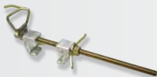
3091 - HLL Bypass Beam Clamp fits 4" - 16 5/8" width 1/4" - 1 3/4" thick (4 - 41.5cm width .6 - 4.4cm thick)
