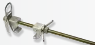
3093 - HLL Anchorage Beam Clamp fits 4" - 16 5/8" width 1/4" - 1 3/4" thick (4 - 41.5cm width .6 - 4.4cm thick)
